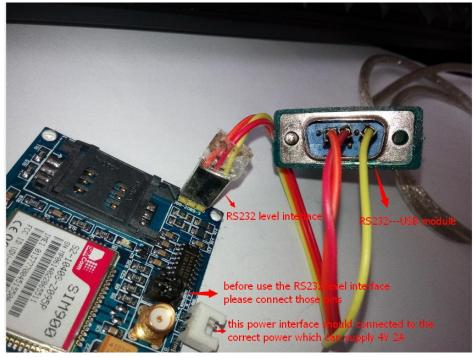
You can connect the sim900 module with the PC using a USB—TTL moudule as shown below.
