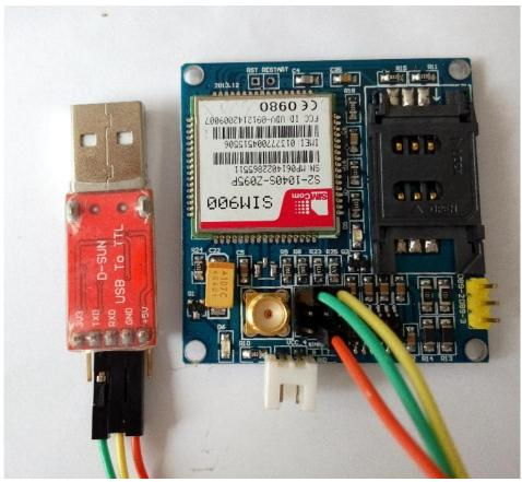
Plese notice that the power supply voltage should be 3.7-4.2V and it can provide 2A or more
