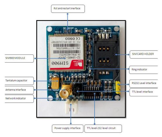
Before you use the RS232 level interface, please connect the four pins as the shown below.
